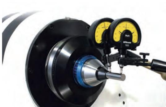
Setup - Concentric with the machine
